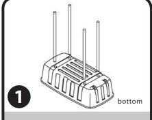
Remove straps, open trunk and remove parts. Turn trunk bottom upside down. Push legs into holes located on the trunk bottom.
