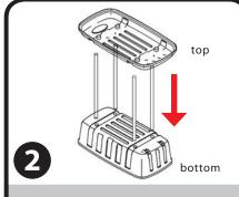
Place trunk top above legs. Align legs with holes in trunk top. Push trunk top down to firmly anchor on legs.
