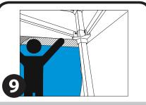
Continue attaching the fastener all the way to the end until the full wall is totally adhered to the canopy.
