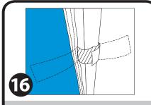
Attach the fastener around each leg on either side of the half wall.
