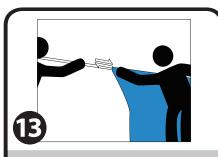
Slide the steel connection bar through the pole sleeve of the half wall.
