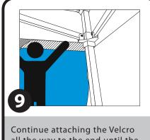
Continue attaching the Velcro all the way to the end until the full wall is totally adhered to the canopy.
