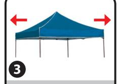
Expand the frame out fully by having each person stand on opposite sides, grasping the outer legs, lift up and step backwards at the same time until tent is fully opened.
